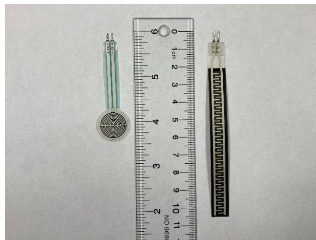
Fig. 3: Geometries and sizes of two flexible force/pressure sensors used in this study.
