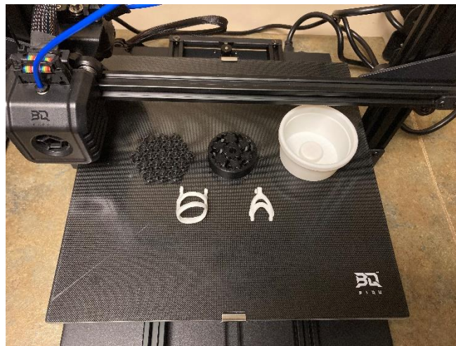
Fig. 6: Fixtures of different polymer materials with different geometries and sizes fabricated with the 3D printing systems in this study.
