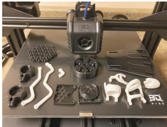
Fig. 12: Fixtures of different geometries and sizes fabricated with the 3D printing technology for robotics applications in this study.
