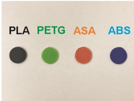
Fig. 1: 3D printed discs of PLA, PETG, ASA and ABS for hardness measurement.
