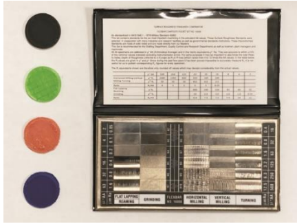
Fig. 10: Evaluation of the surface roughness of a sample with a standard set (FLEXBAR Model No. 16008).
