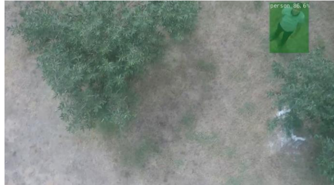
Fig 9. Detection of lost persons in the search area using SSD-Mobilenet-v2 and detectNet classes.
