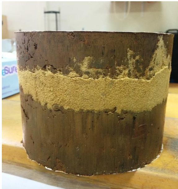
Fig. 1: One of the position of sandy layer in Proctor mould after compaction.
