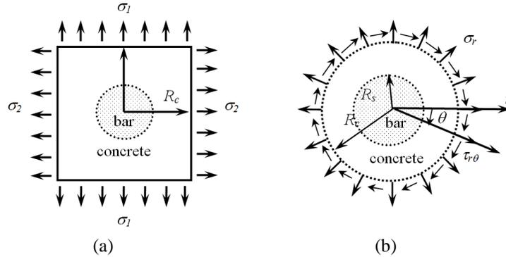
Fig. 1: Planar stress state of the plain round bar embedded in concrete subjected to lateral tensile stresses: (a) under principle stress axes; (b) under polar axes.
