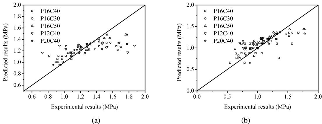
Fig. 4: Comparison between predicted and experimental ultimate bond strength under: (a) uniaxial tensile stress; (b) biaxial tensile stresses.
