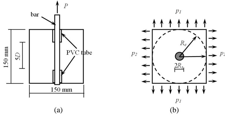
Fig. 3: Schematic of the pull-out specimen: (a) cross-section view; (b) top view and the lateral tensile stresses.
