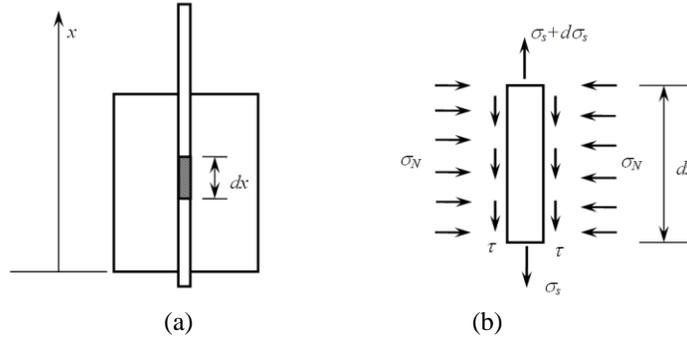
Fig. 2: Schematic of stress analysis for pull-out process: (a) the pull-out specimen; (b) the element of the bar.
