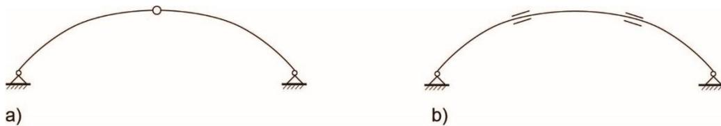
Fig. 20: Suitable placing of joints in arch structures. a) three-hinged arch; b) two-hinged arch.
