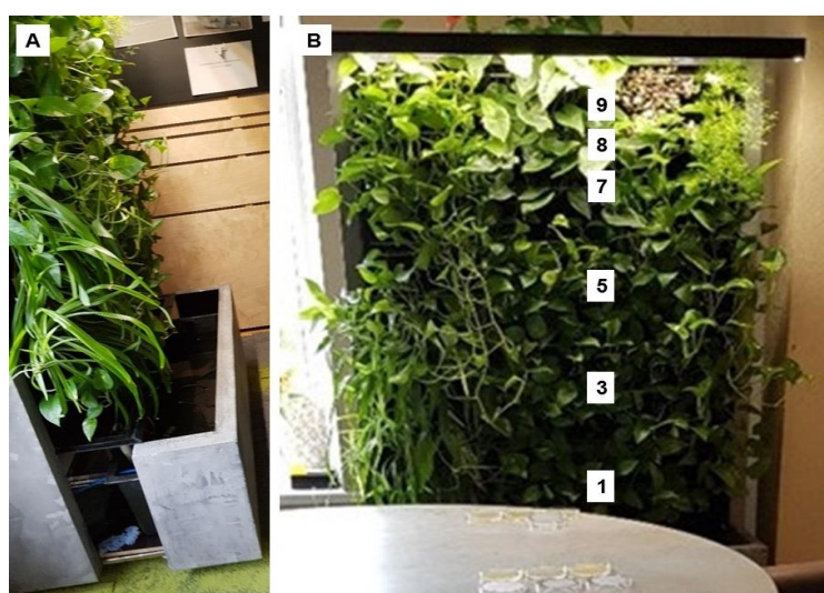
Fig. 1: The experimental green wall established in the office room. A – side view; B – frontal view with the numbered levels, where ceramic granules have been sampled.
