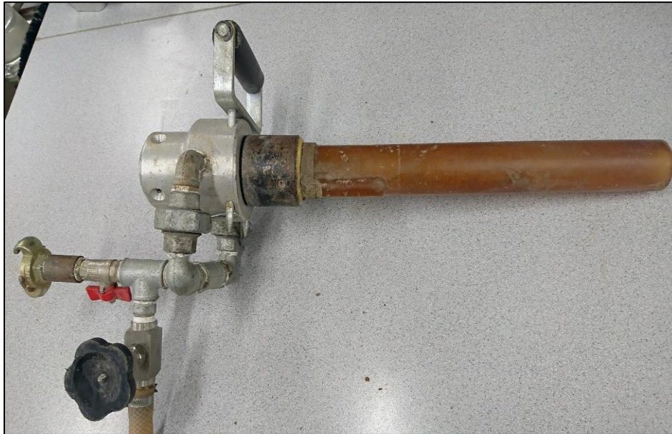
Fig. 4: Nozzle used for the application of bentonite on experimental dam.
