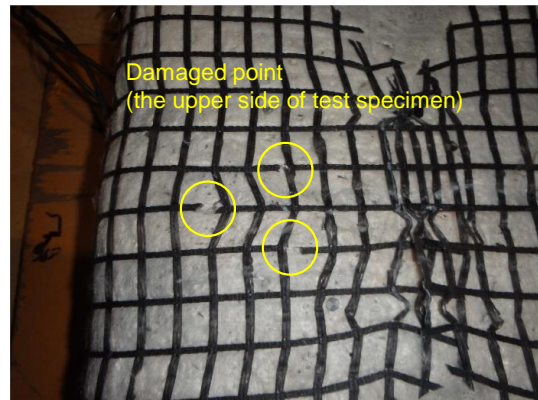
(b) Damaged points of geotextile
