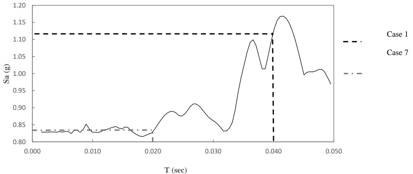
Fig. 5 Acceleration response spectrum (5% damped) of the Pedernales-Ecuador earthquake, April 2016 and spectral values for the third vibration mode, Cases 1 (wet) and 7 (dry) finite element models.
