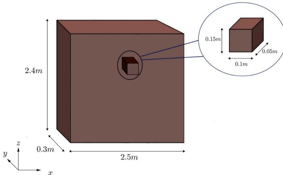
Fig. 1 Geometry of the rammed-earth wall finite element model
