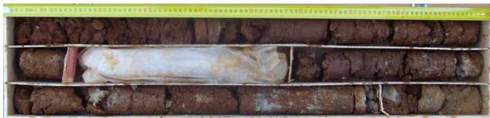
Figure 2: Drilled coring in volcanic weathered basalt.
