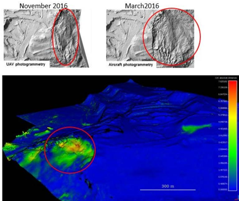
Fig. 4: The two different orthophotos (November 2016 and March 2017) of the western slope (above) and cloud to cloud comparison (down) between two different DEM (November 2016 and March 2017). Red circle indicates the ground movement in m occurred over 3 months.
