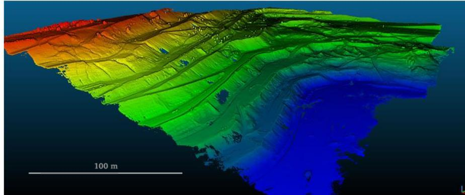
Fig. 3: height-colored point cloud from the LiDAR acquisition (red 200m altitude and blue -30m altitude).
