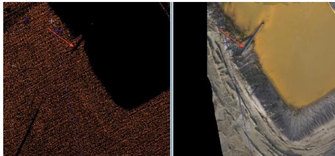
Fig. 6: to the left point density variation related to the material nature (water and dark pipes) shown on the orthophoto to the right.
