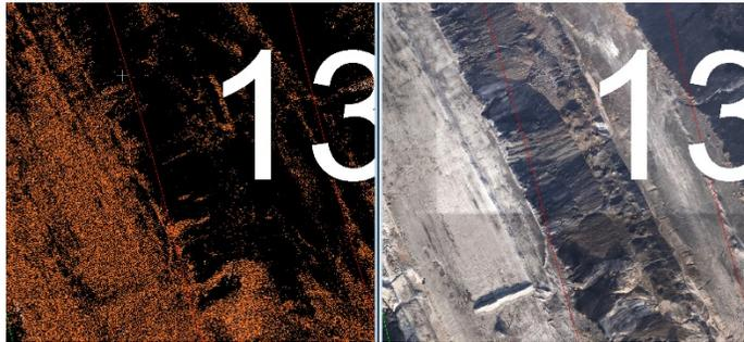
Fig. 5: to the left point density variation related to material nature (coal) shown on the orthophoto to the right.
