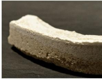
Figure 4: Surface treatment using MICP
