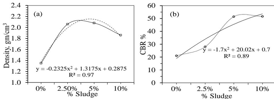
Fig. 7: Change in % sludge versus: (a) density; and (b) CBR%
