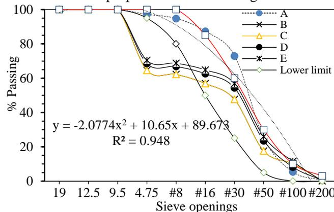
Fig. 1: Particle size distribution according to ASTM C33
