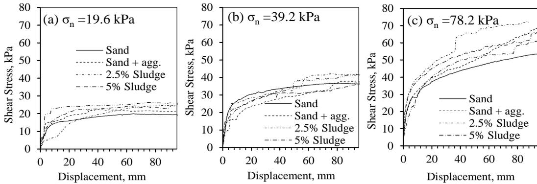
Fig. 3: Shear-displacement at normal stresses: (a) 19.6; (b) 39.2; and (c) 78.2 kPa
