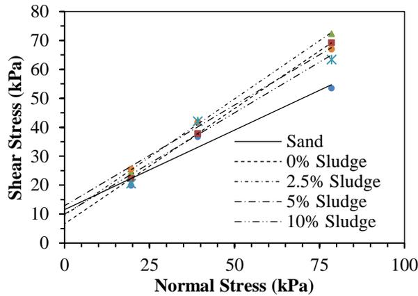
Fig. 4: Shear failure envelopes for the five test samples
