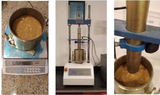
Fig. 6: CBR samples preparations and load test machine
