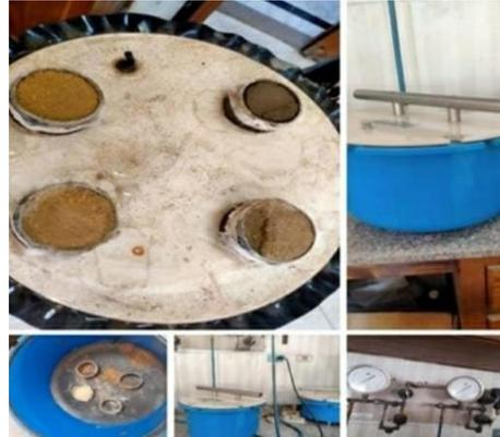
Fig. 8: Pressure membrane test device and components
