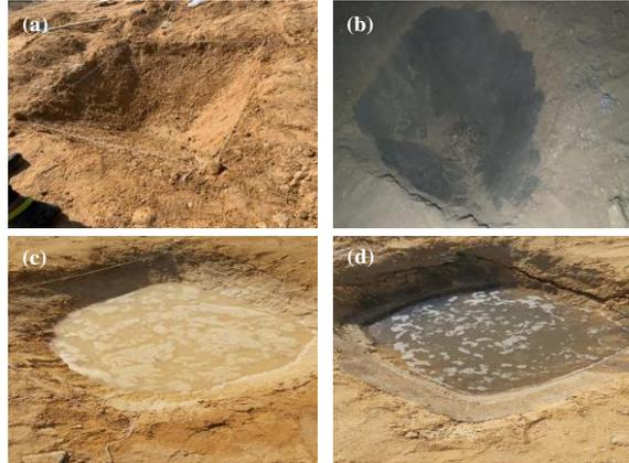
Fig. 9: (a) sand pit; (b) sludge pit; (c) sand pit with water; and (d) sludge pit with water
