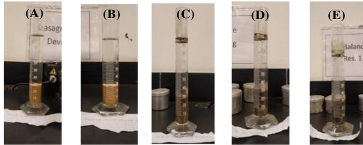
Fig. 2: Free swelling test on all samples
