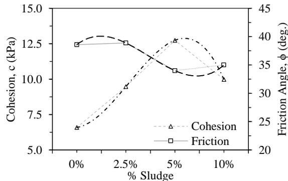
Fig. 5: Change of shear strength vs. percentage of sludge in the mix
