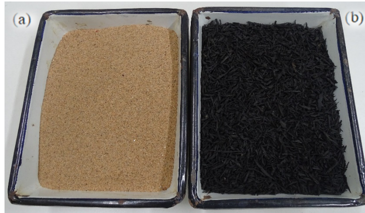
Fig. 1a-b: Fill material used in the study (a) Sand; (b) Crumb rubber
