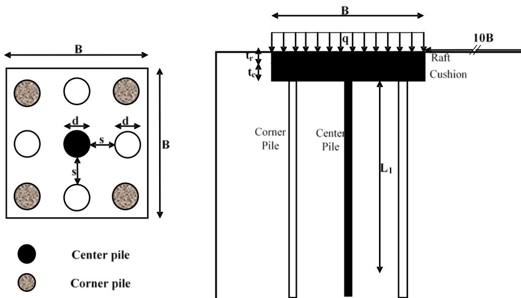
Fig. 1: Schematic Representation of the DPR system model
