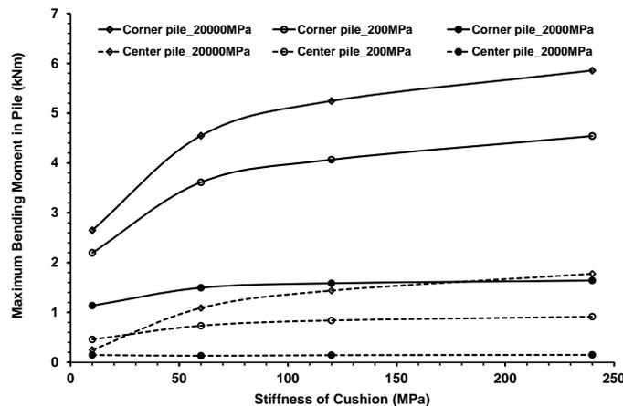
Figure 5: Variation in maximum bending moment in the system of piles in the DPR system due to change in cushion and pile stiffness
