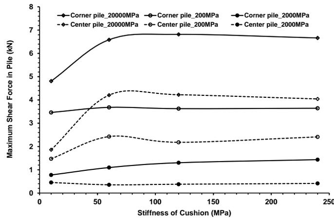
Figure 7: Variation in maximum shear force in the system of piles in the DPR system due to change in cushion and pile stiffness
