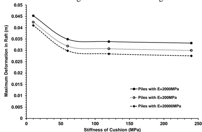
Figure 2: Variation in maximum deformation/settlement at the centre of the raft of DPR system due to change in cushion and pile stiffness
