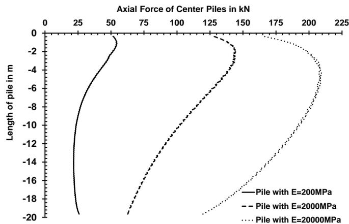
Figure 8: Variation in axial force distribution along the length of piles in the DPR system due to change in pile stiffness
