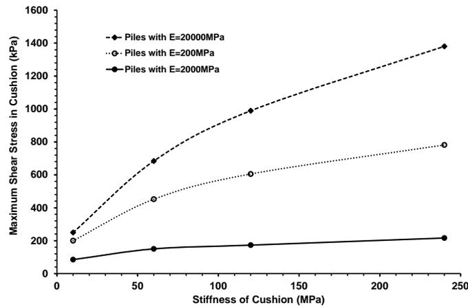
Figure 3: Variation in maximum shear stress in the cushion layer of DPR system due to change in cushion and pile stiffness
