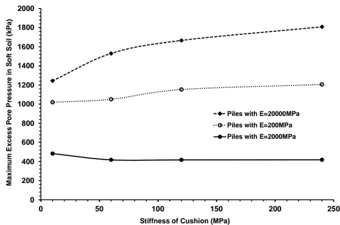
Figure 4: Variation in maximum pore pressure generation in the soft soil layer of DPR system due to change in cushion and pile stiffness
