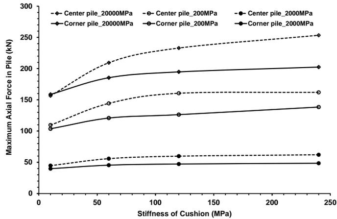
Figure 6: Variation in maximum axial force in the system of piles in the DPR system due to change in cushion and pile stiffness
