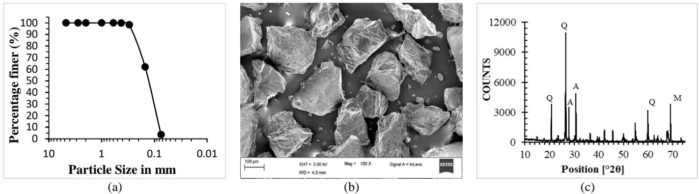
Fig. 1 (a). Grain Size Distribution Curve, (b). SEM micrograph, and (c). XRD plot of the Brahmaputra riverbank sand.
