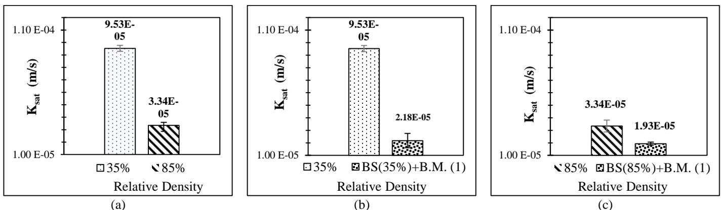
Fig. 4 Comparison of average saturated Hydraulic conductivity of the untreated and treated sand at (a). Different densities, (b). Loose state (untreated and treated), and (c). Dense state (untreated and treated).
