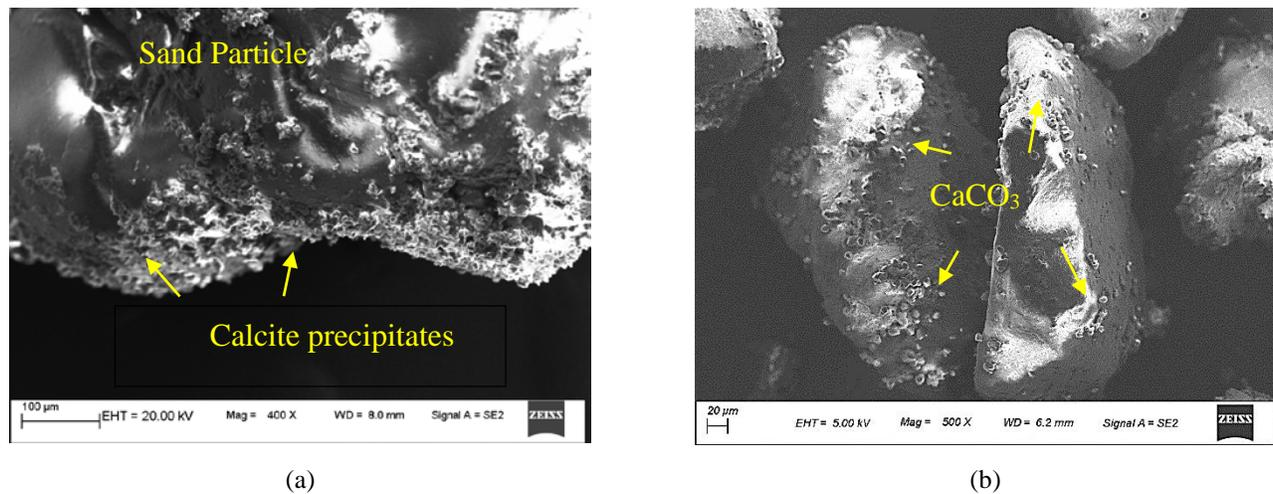
Fig. 5 (a). The precipitated calcite over sand surface, and (b). sand grains without bridging.
