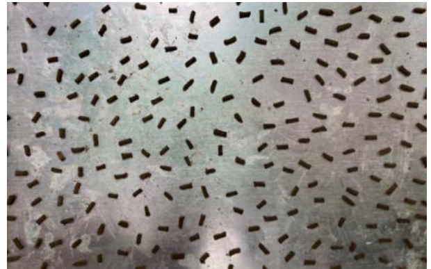
Fig. 2: Three millimetres (3 mm) diameter cylindrical shape 'green' granules.
