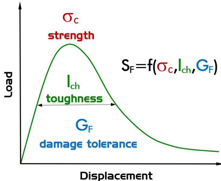
Fig. 2: Schematic illustration of the structural safety factor principle [16]. Picture Credit: FRACTURE ANALYTICS
