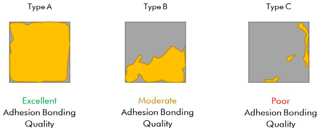
Fig. 1: Overview of three basic types of adhesion bonding quality. Picture Credit: FRACTURE ANALYTICS
