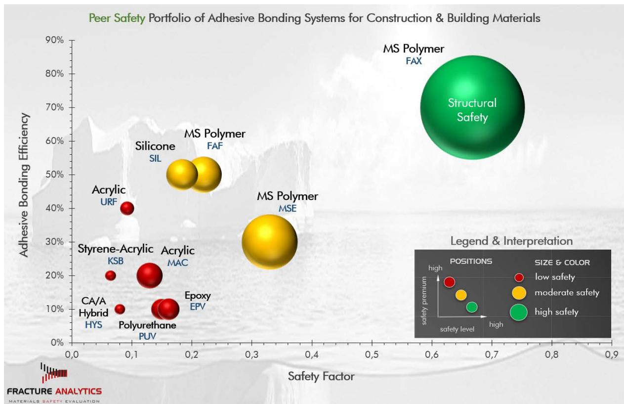
Fig. 4: Peer safety portfolio of adhesives systems used for concrete bonding. Picture Credit: FRACTURE ANALYTICS
