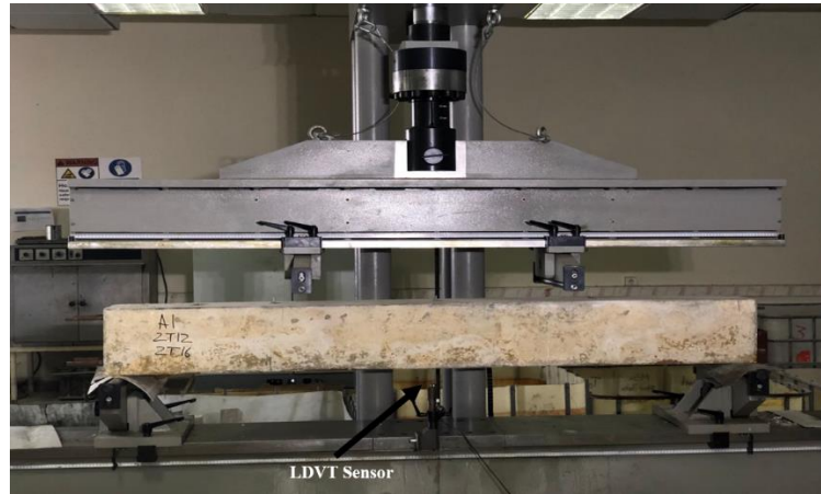
Figure 5: Four-point loading test performed on beam A1
