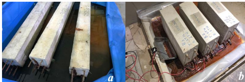
Figure 3: Experimental set-up where (a) A1 (b) B1 are placed at the end of current exposure
