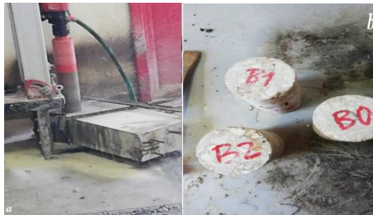
Figure 6: (a) Coring test performed on beam (b) Cores Extracted
