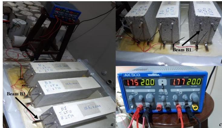
Figure 2: (a) Experimental setup of accelerated corrosion of reinforced concrete beams with B1 inside, (b) connection between beams, (c) power source providing DC current
