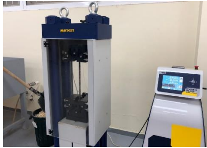
Figure 7: Tensile test performed on extracted corroded steel
