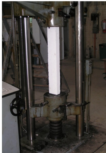
Figure 1: (a) Detailing of test specimens, (b) Tensile loading test setup
