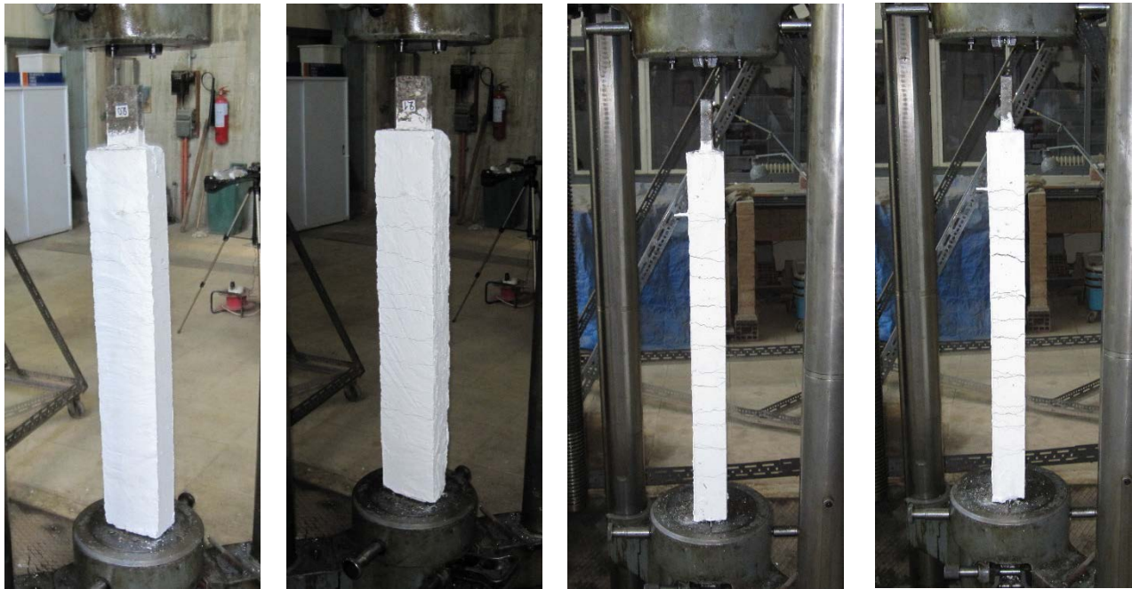
Figure 2: Shape of specimens tensile strain: (a) COLUMN-1, (b) COLUMN-2, (c) COLUMN-3, (d) COLUMN-5
