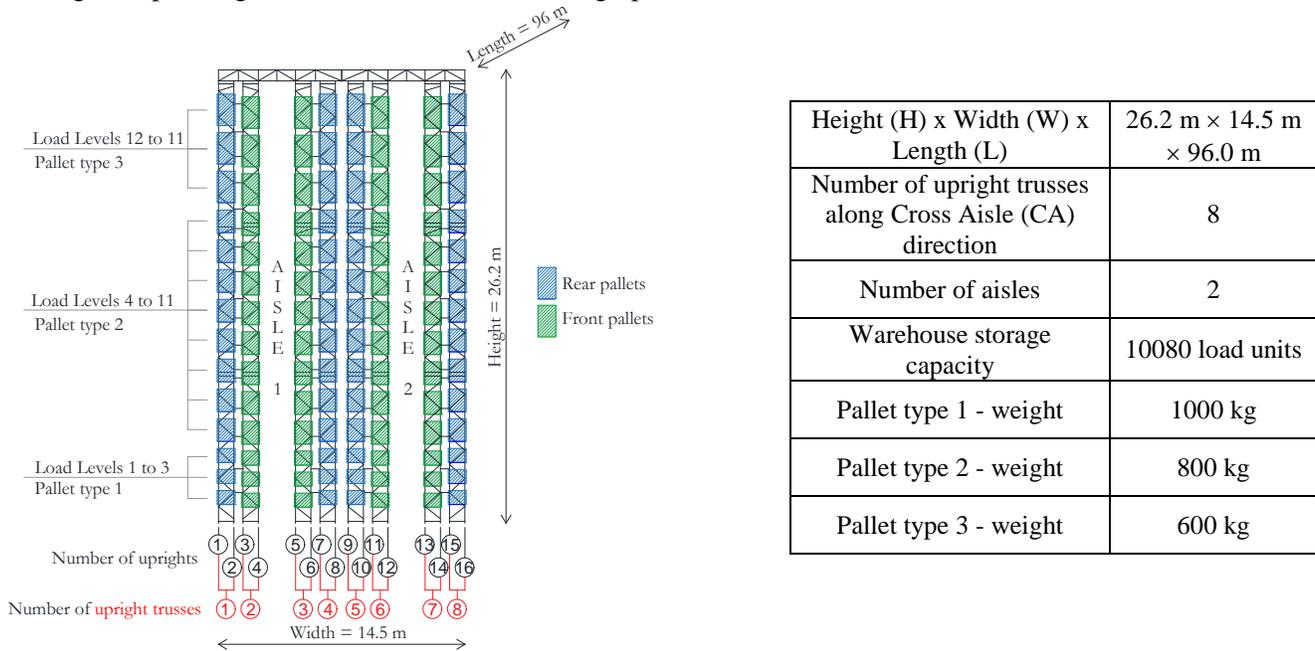
Figure 1: Definition of some of the design input parameters for the case studies.
