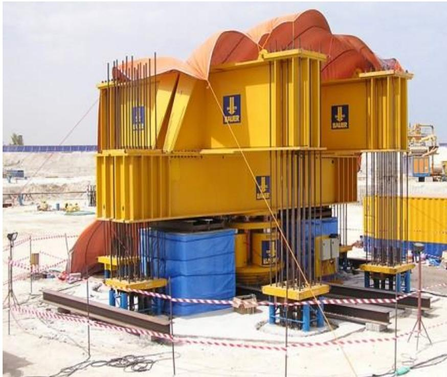
Fig.1: Static compression pile load test setup
