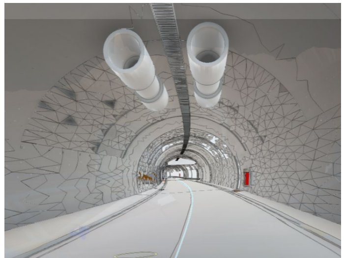
Fig. 10: View of the final Coordinated Model on the CDE (BIMCollab), seen from the interior of Kolltveit tunnel.
