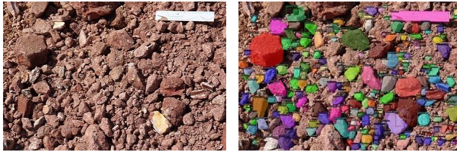
Fig. 4. Image input to the model and the predicted image containing segmentation masks.
