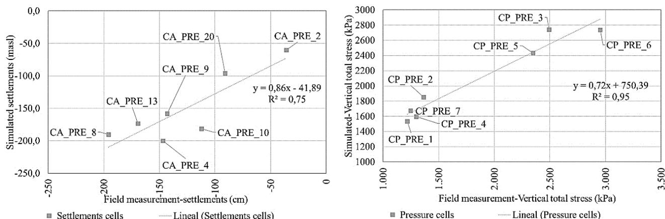
Fig. 10: Level of correlation between core settlement readings (left side) and total vertical core stresses (right side) with numerical modeling.
