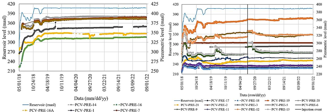
Fig. 5: Historical records of piezometers located in the core below 385 m.a.s.l (left side) and foundation (right side).
