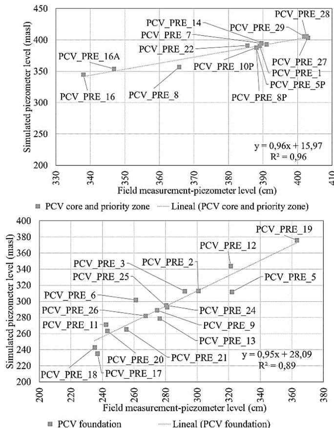
Fig. 9: Level of correlation between piezometric field readings in the dam fill (left side) and foundation (right side) with numerical modeling.
