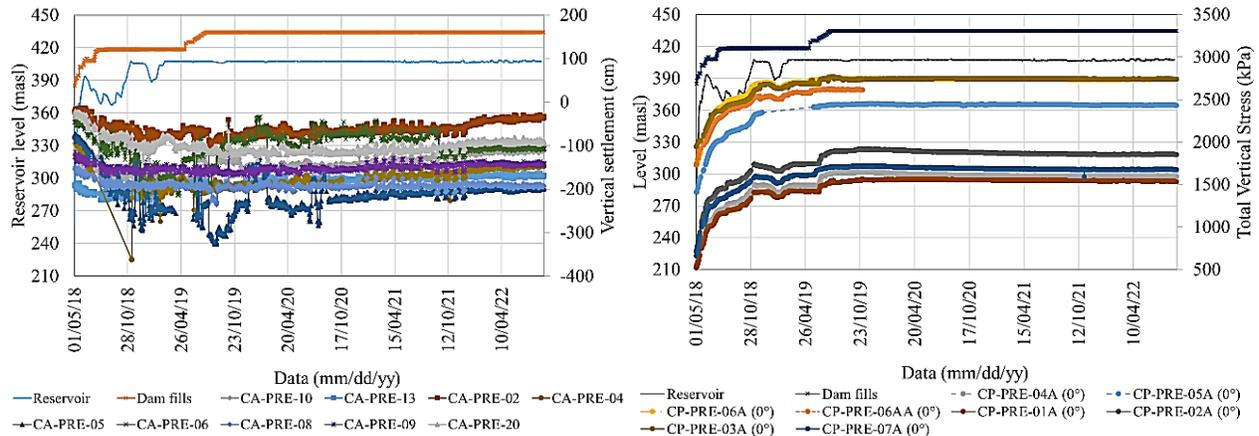
Fig. 7: Historical records of settlement cells (image on the left) and vertical pressure-stress cells (image on the right).
