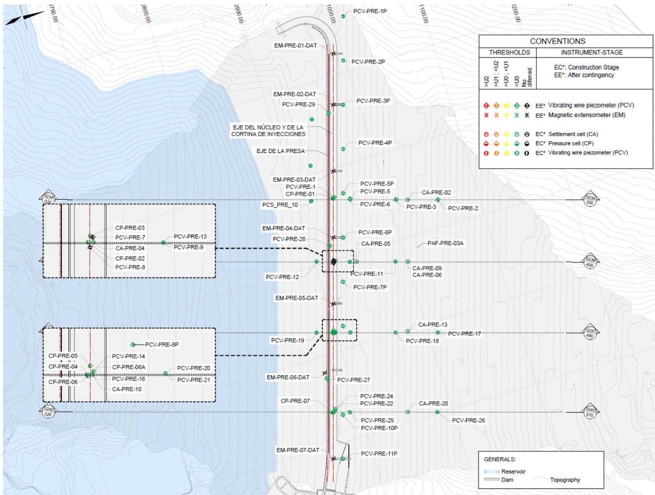
Fig. 3: Instrumentation of the Ituango dam- piezometers.
