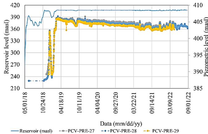
Fig. 6: Historical records of piezometers on the upstream side of the cutoff wall.
