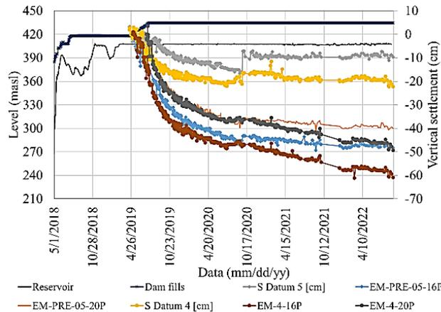
Fig. 8: Historical record of magnetic extensometers 4 and 5 (the datum sensor corresponds base of the cutoff supported by the lower core 1A, the 16P sensor corresponds to the plate closest to the cutoff-upper core transition 1A and, the 20P sensor represents the plate closest to the crest of the dam).
