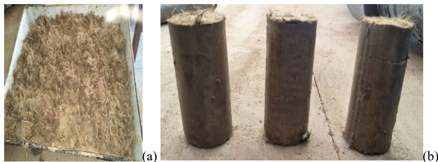
Fig. 2: Sample preparation for (a) Compaction test and (b) UCS
