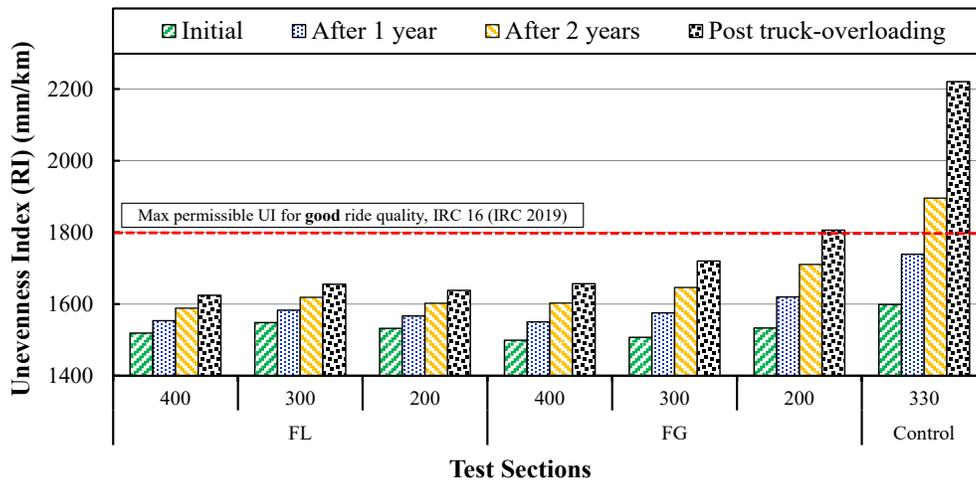
Figure 3. Summary of Unevenness Index using fifth wheel Bump Integrator.
