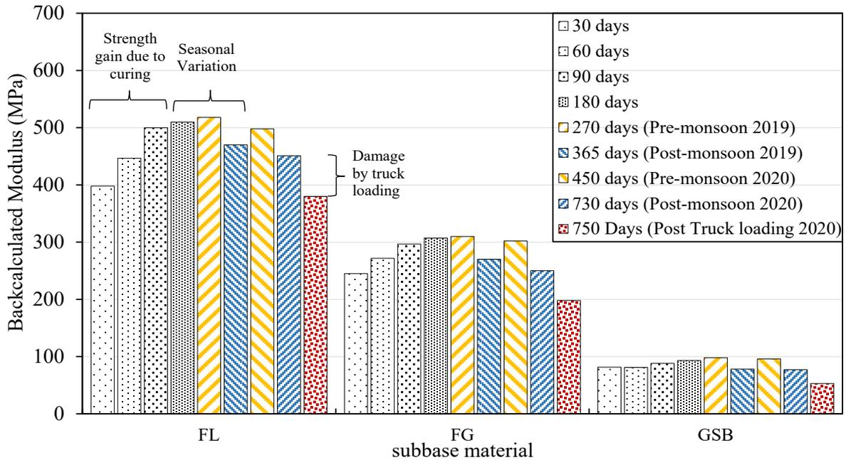
Fig. 2: Change in Backcalculated moduli values of FL, FG and GSB layers with curing period
