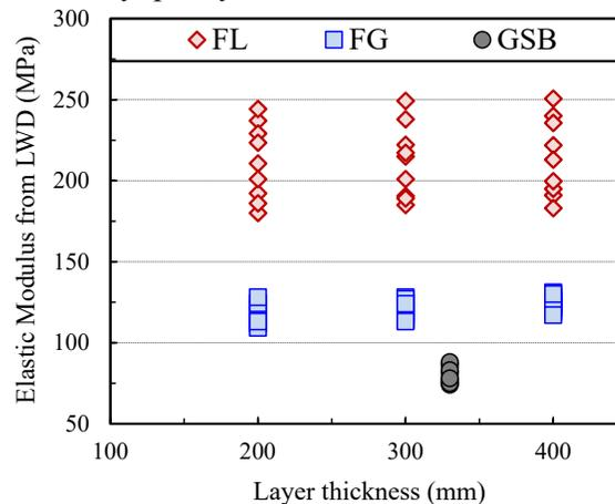
Figure 1. LWD modulus of FL, FG and GSB layers recorded 7-day post-construction.
