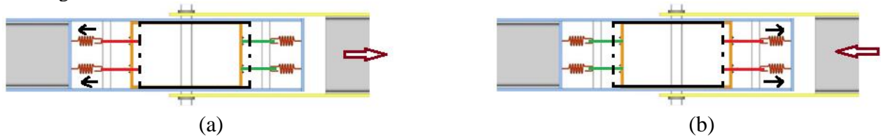
Figure 2: Shape Recovery Force SRF in SMA springs of semi-active SMA-TSD (a) Right sway position (b) Left sway position
