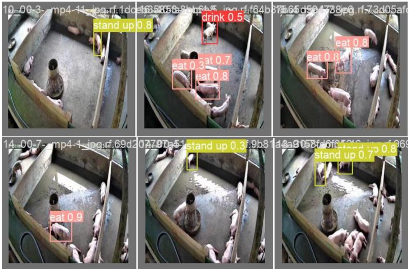
Fig. 2: Example of detecting pig postures using YOLOv8 model.
