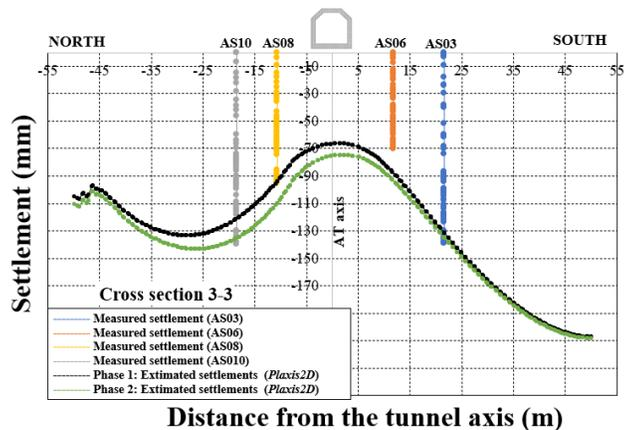
Fig. 6: Comparison between predicted settlement after pre-load phase 1 (black dotted line) and pre-load phase 2 (green dotted line) with measured settlements: a) cross section 1-1; b) cross section 2-2; c) cross section 3-3.
