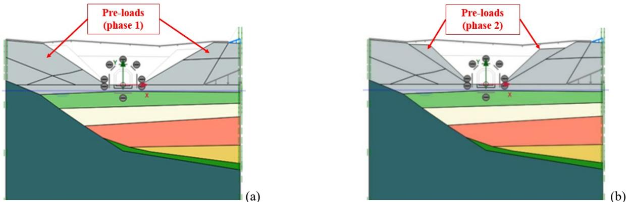
Fig. 3: Section 2-2, pre-loads in FE *Plaxis2D* models: a) phase 1; b) phase 2.
