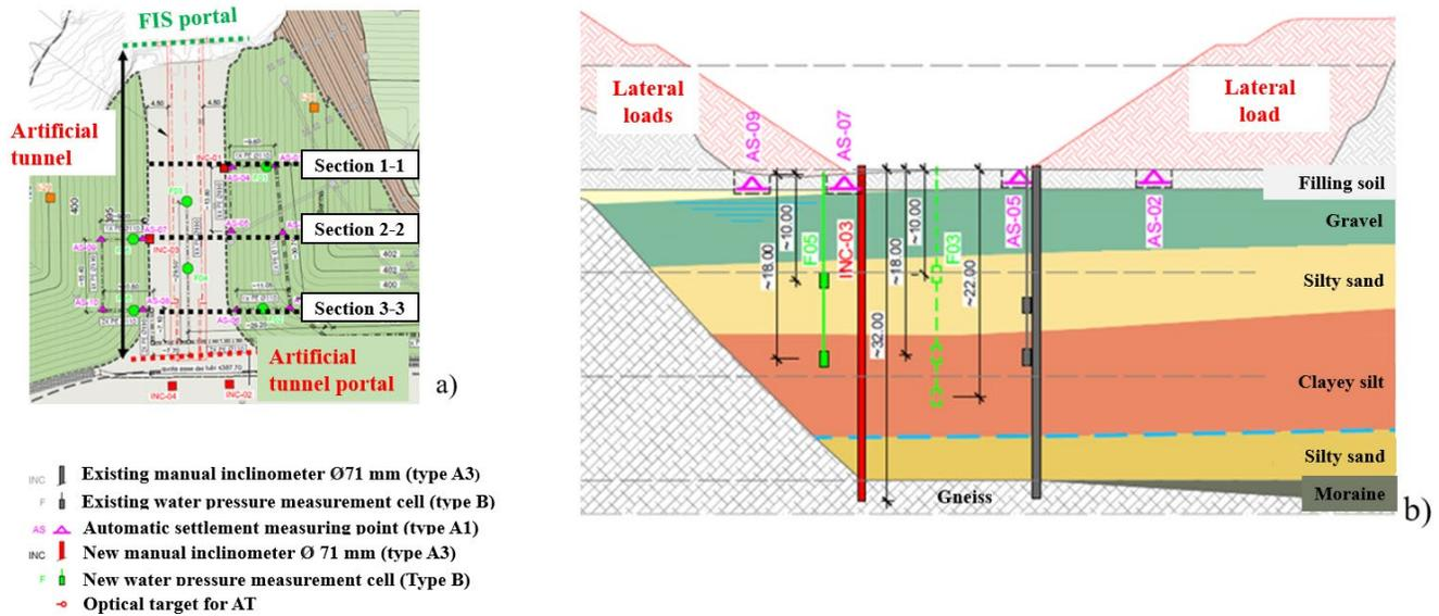
Fig. 4: a) Plan view of the artificial tunnel; b) cross-section 2-2 and instrumentation.
