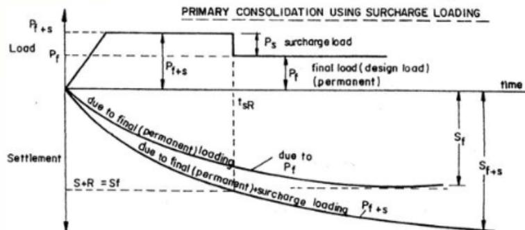
Fig. 1: Primary consolidation using surcharge loading.
