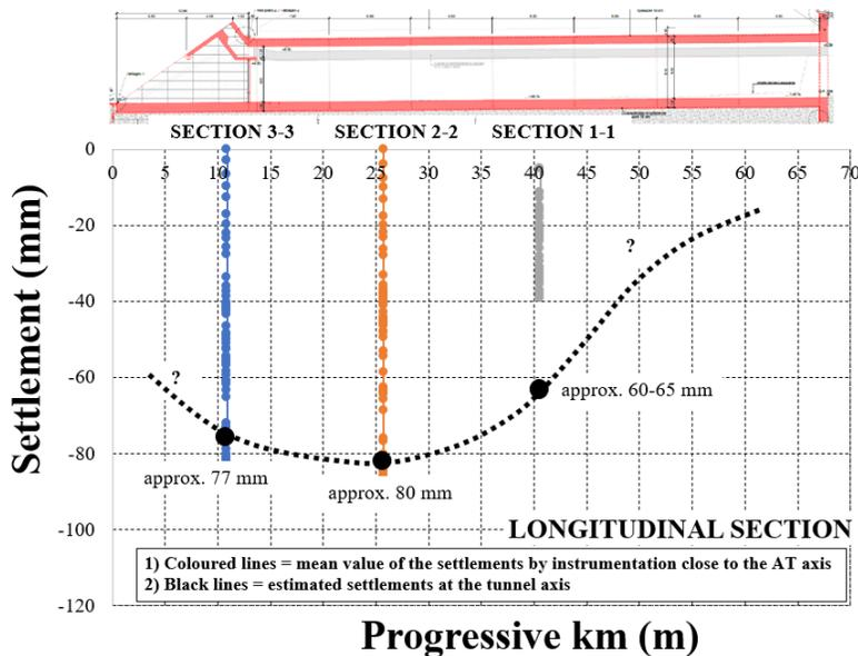
Fig. 7: Longitudinal section of the tunnel axis: monitored settlements of cross sections 1-1, 2-2, 3-3 (coloured vertical lines) and estimation of the settlement distribution along the longitudinal direction (dotted black line).
