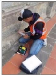
Fig. 4 Sclerometer test.
