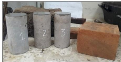
Fig. 4 Rock Cores and Brick Block.
