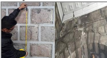
Fig. 1 Measurement of cracks in the Church.
