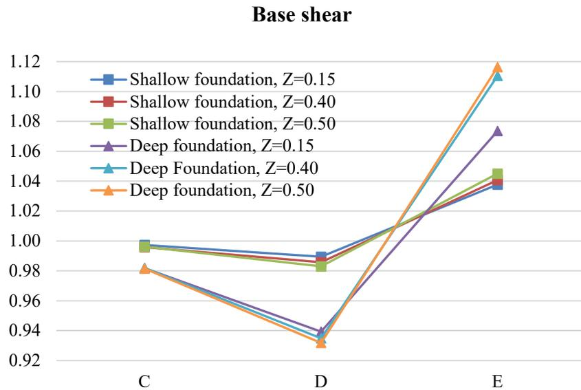
Fig. 4: Base shear and moments ratios of the SSI model to the fixed model
