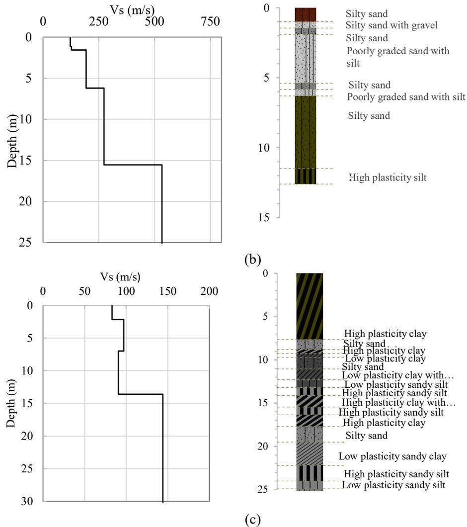
Fig. 3: Ground wave velocity and stratigraphy: (a) Soil type C, (b) type D, (c) type E
