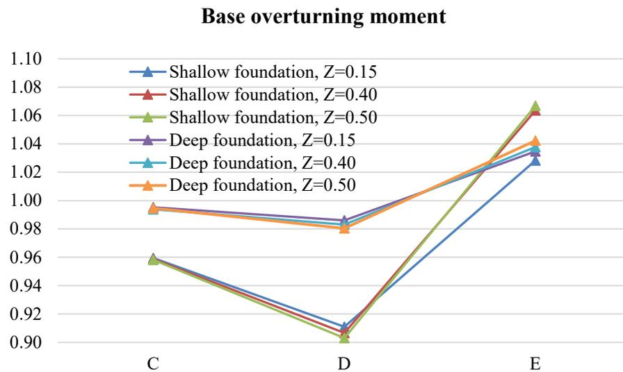
Fig. 5: Base shear and moments ratios of the SSI model to the fixed model
