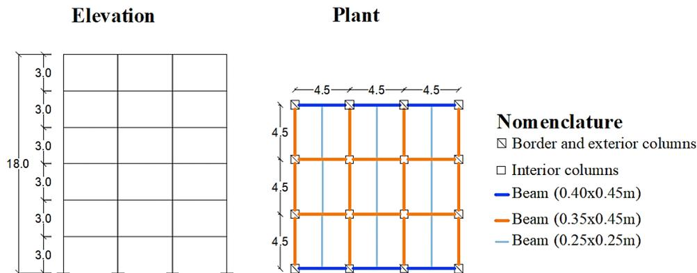
Fig. 1: Elevation and plant configuration of building type.
