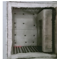
Fig.4. Frame specimen inside the furnace
