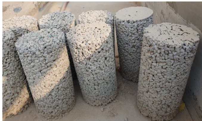
Fig. 3: Pervious concrete samples ready for testing.
