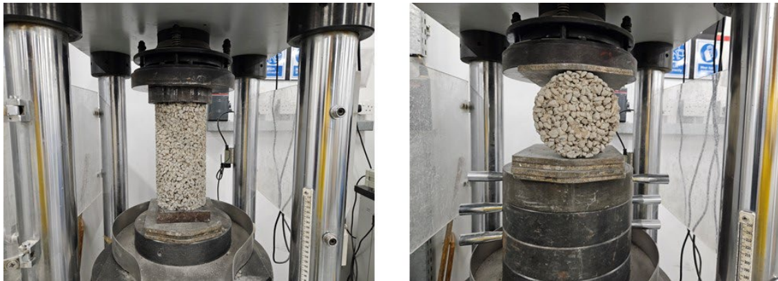
Fig. 4: Determination of compressive and split tensile strengths of pervious concrete.
