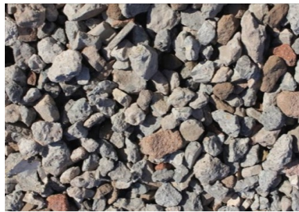
Fig. 1: Recycled coarse aggregate produced by Beeah, UAE, and used in the study.
