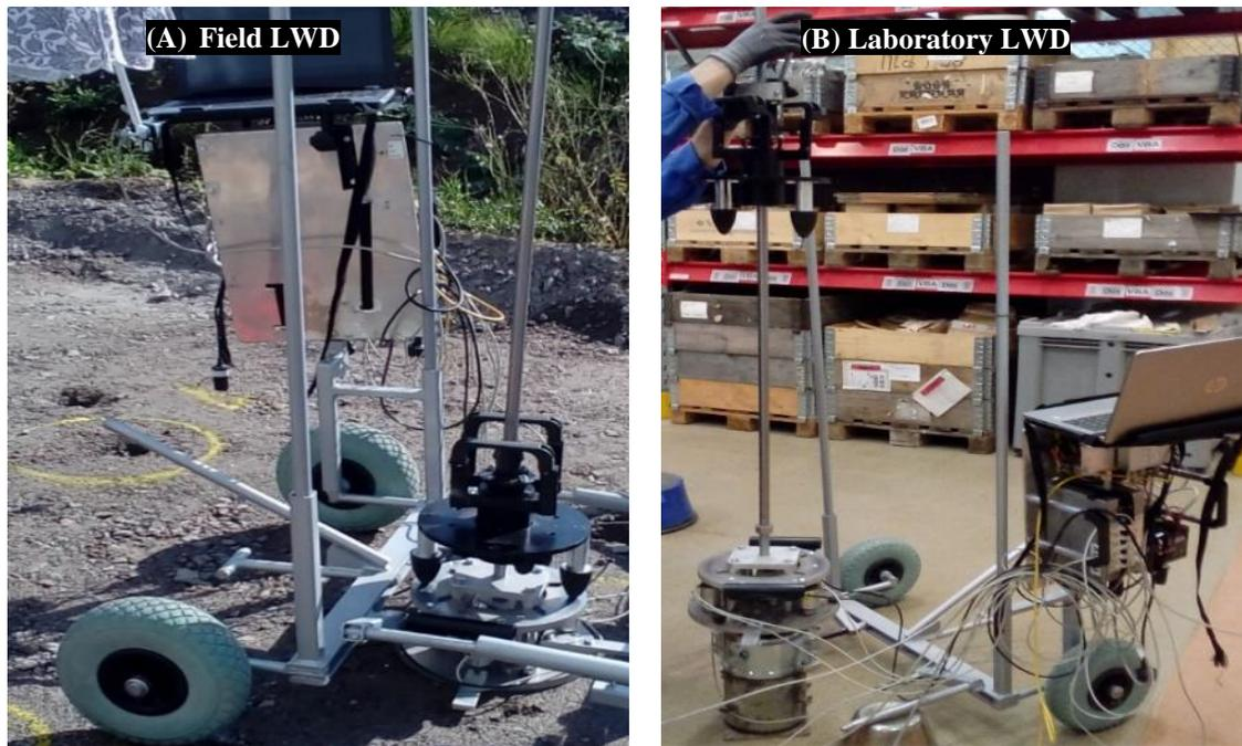
Fig. 1: Field (A) and Laboratory (B) LWD testing on unbound base material.
