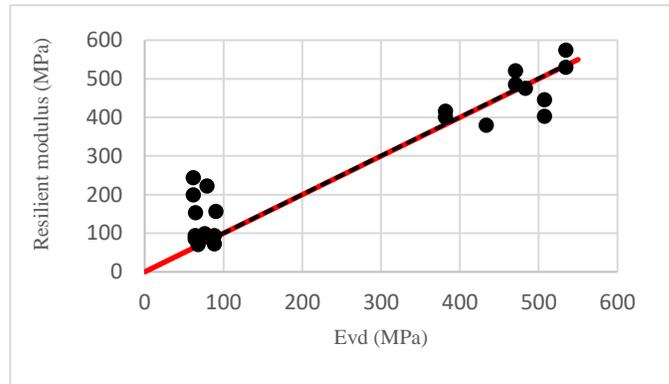
**Figure 2:** Correlation between the measured resilient moduli and dynamic deformation moduli
