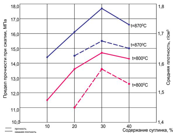
Fig. 1. Strength and average density of brick depending on the content of mechanically activated loam
