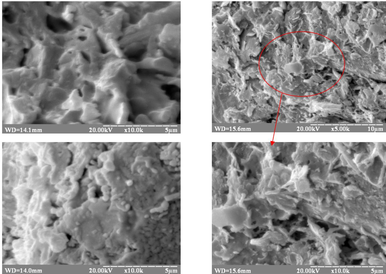
Fig. 8. Microstructure of samples fired at 870 °C, made from complex-activated raw materials of the following composition, wt. %: coal enrichment waste – 70; loam – 20; red mud – 10
