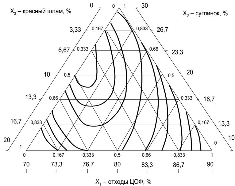
Fig. 2. The diagram of the state "composition – compressive strength" of wall ceramic samples of the studied system
