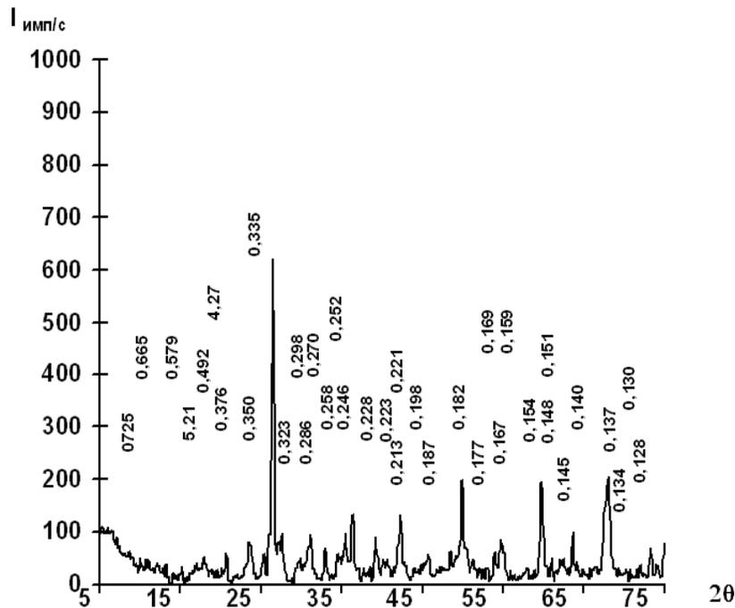
Fig. 5. Diffraction pattern of a sample fired at 870 0C, with the following composition, wt. %: coal
