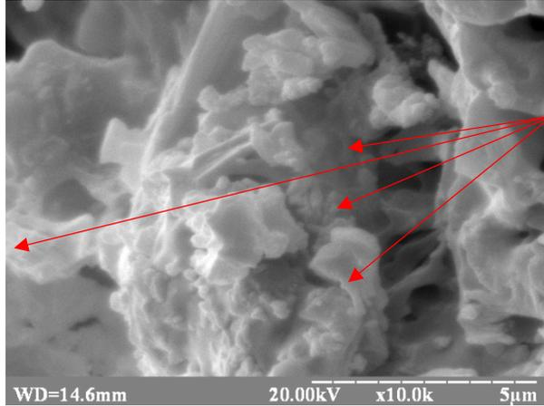
Fused bridges that unite mineral particles of different sizes into a monolith
