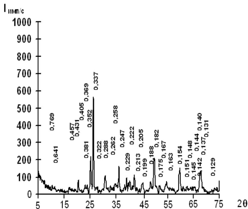
Fig. 4. Diffraction pattern of a sample fired at 870 °C, with the following composition, wt. %: coal enrichment waste – 80; loam – 20
