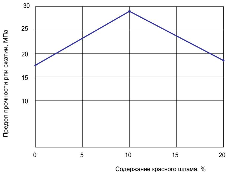
Fig. 3. Dependence of the compressive strength of the material on the content of red mud
