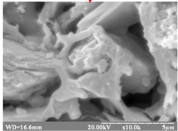
Fig. 7. Microstructure of samples fired at 870 °C made on the basis of a mechanically activated two-component ceramic mass consisting of 80% coal enrichment waste and 20% loam
