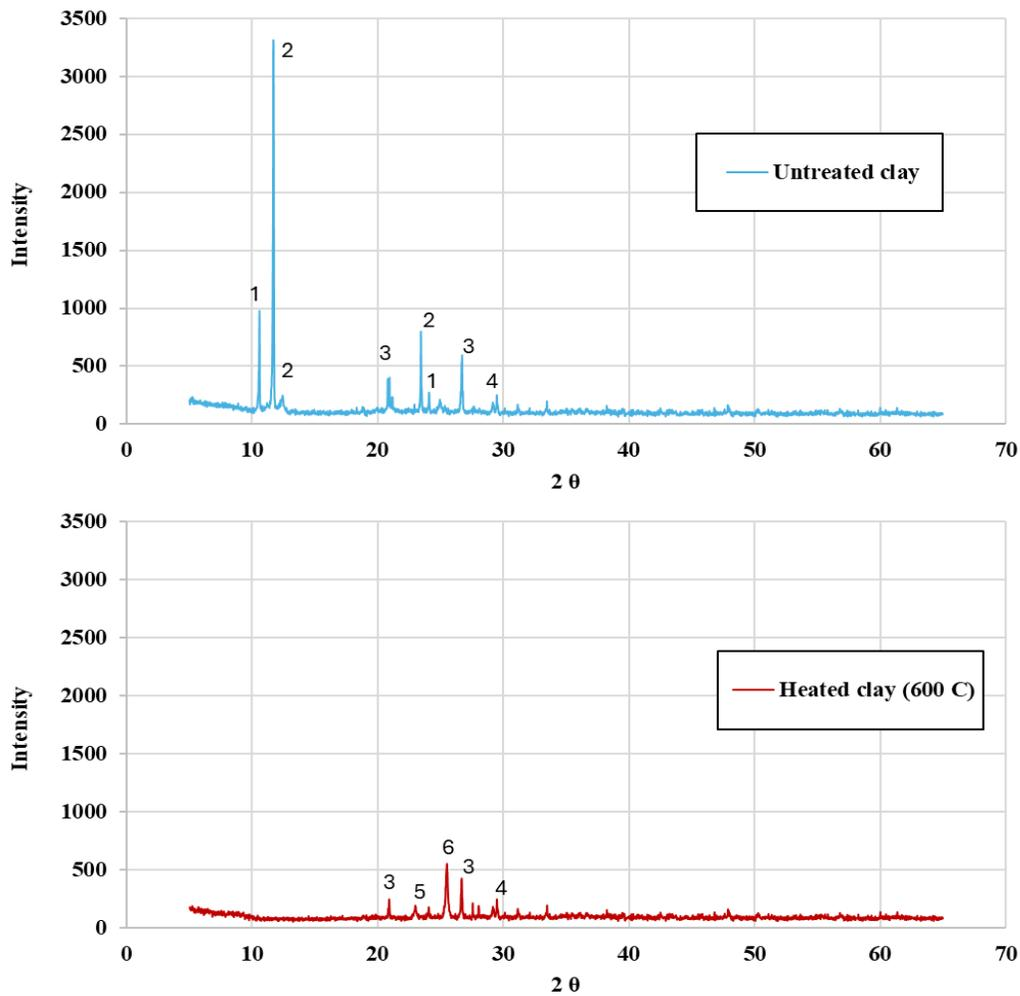
Fig. 5 XRD analysis for untreated clay soil and heated soil under 600 °C for 2 h (1=illite; 2=kaolinite; 3=Quartz; 4=calcite; 5=Dehydrated clay phases; 6=Transformed kaolinite).
