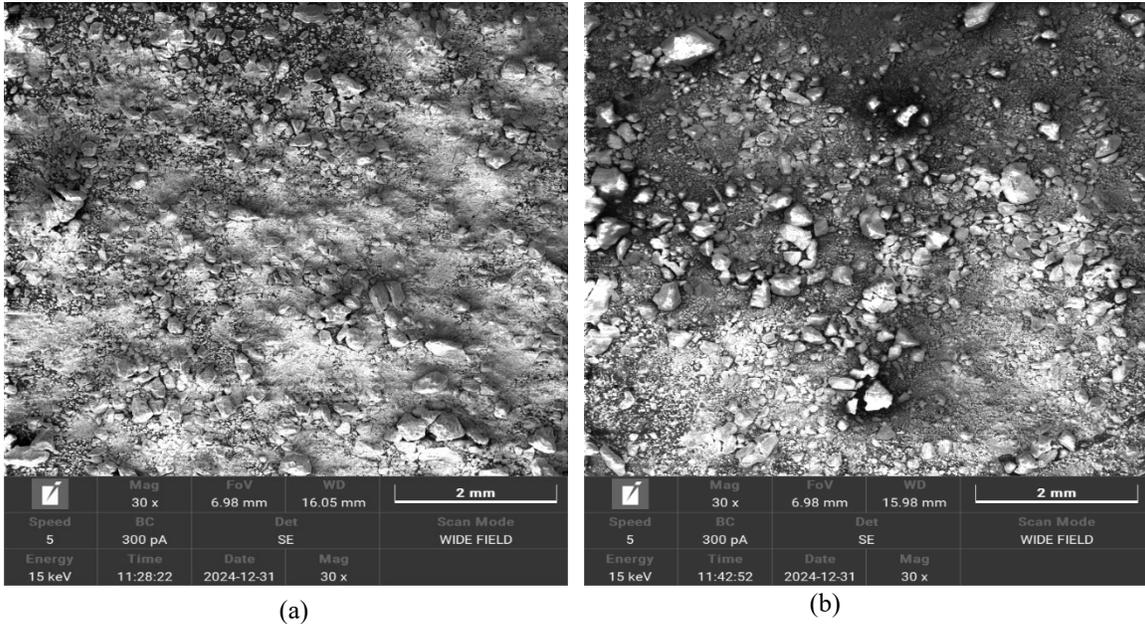
Fig. 3: SEM analysis of expansive clay samples at 30x magnification: (a) Untreated expansive soil; (b) Heated expansive soil (600 °C).
