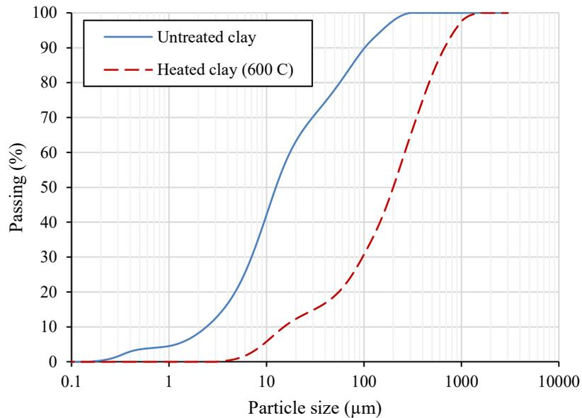
Fig. 2: Particle size distribution (PSD) for untreated and heat-treated expansive soil samples
