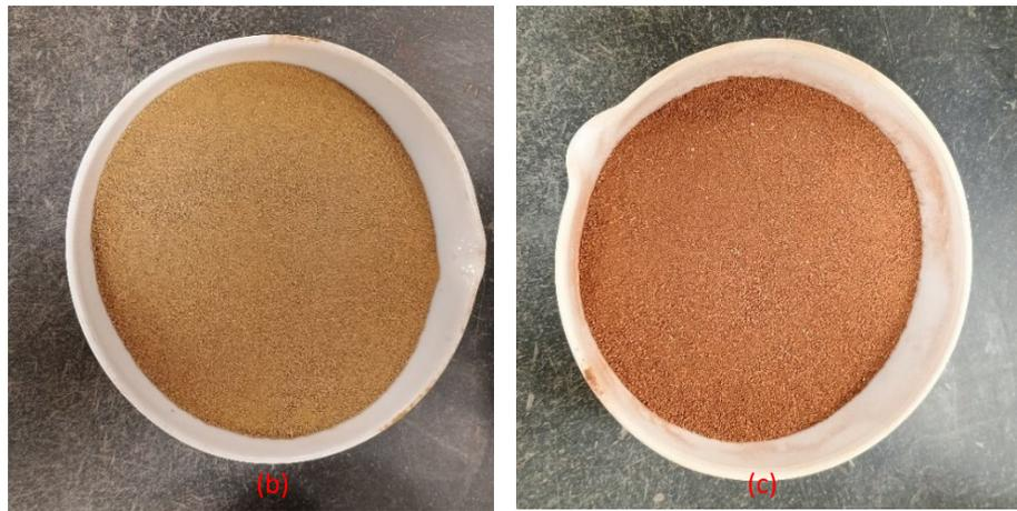
Fig. 1: Procedure of Thermal treatment of expansive soil sample: (a) Electrical furnace; (b) Untreated expansive soil; (c) Thermally treated clay sample.
