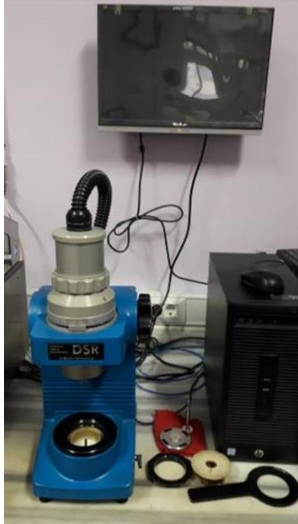
Fig. 1. Dynamic Shear Rheometer (DSR)
