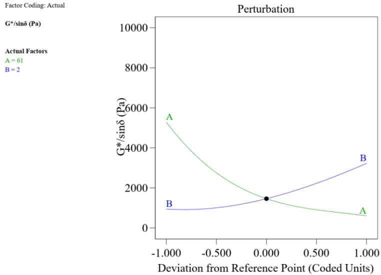
Fig. 3. Perturbation curves for Iraqi bitumen (A:temperature, B:SEBS ratio)
