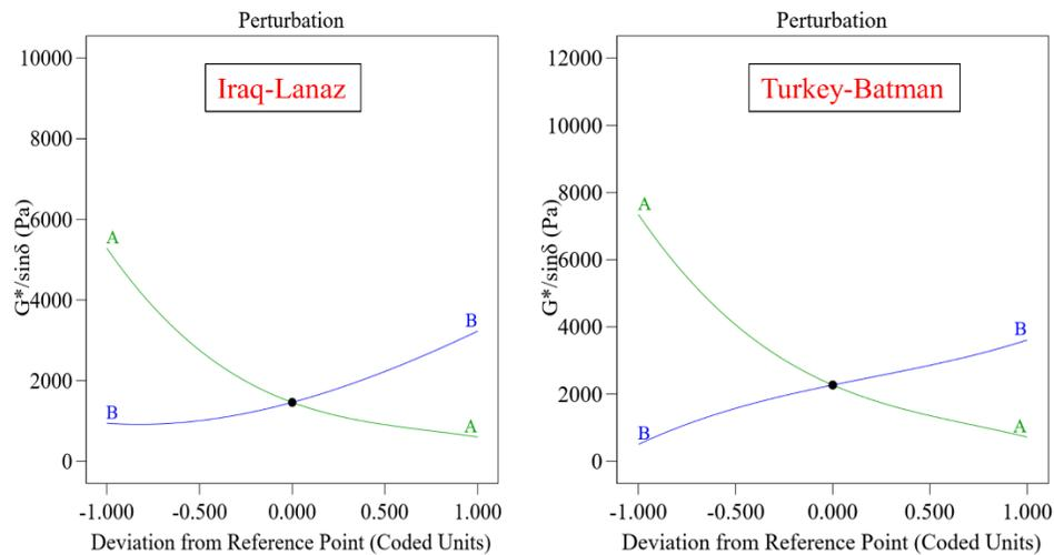
Fig. 6. Comparison of perturbation curves for both bitumen
