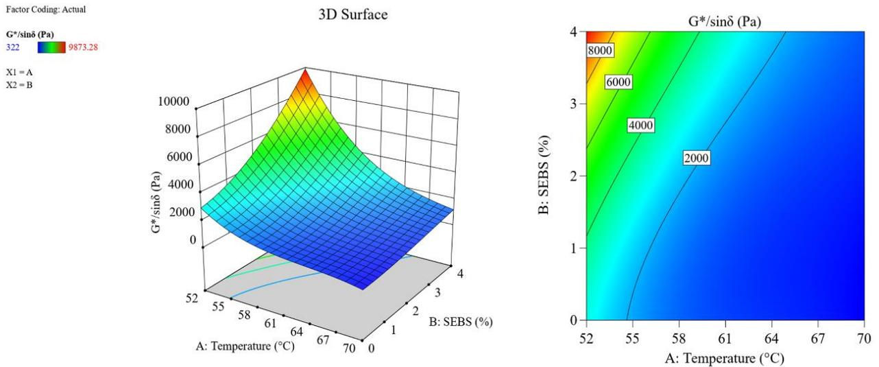
Fig. 2. 2D and 3D RSM plots for Iraqi bitumen
