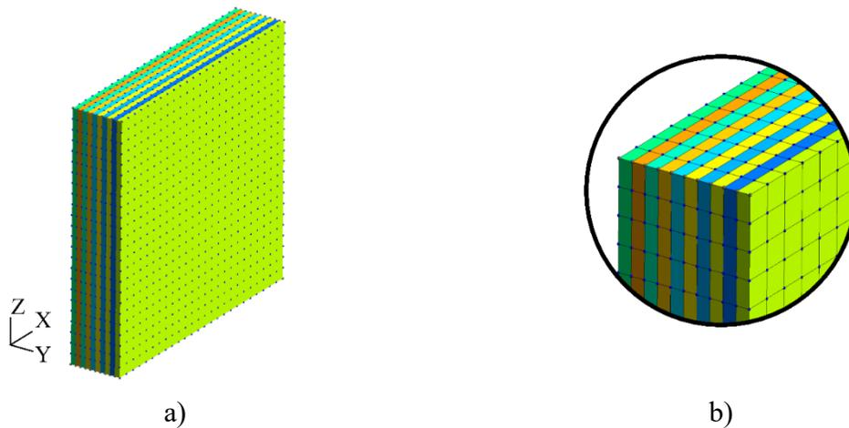
Figure 1: (a) Rammed earth wall FEM model in GMSH and (b) detail of the wall discretization.
