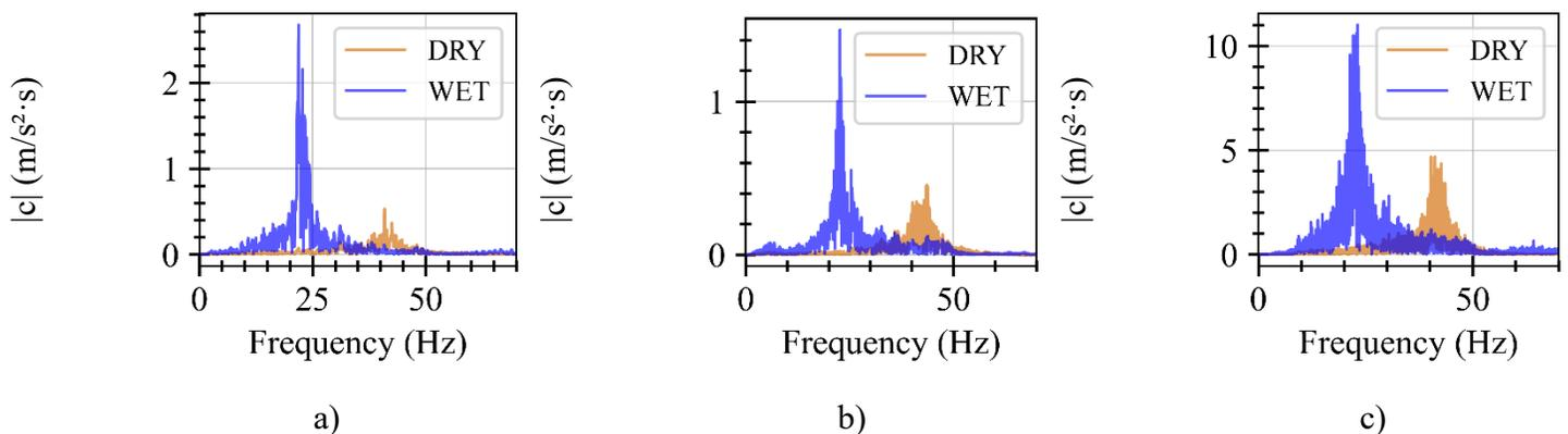
Figure 3: Comparison of FFT between wet and dry conditions for records a) Loma Prieta, b) Chi-Chi and c) Landers.
