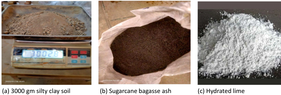
Fig. 1: (a) Soil sample, (b) sugarcane bagasse ash (SBA), and (c) hydrated lime, used in this study.
