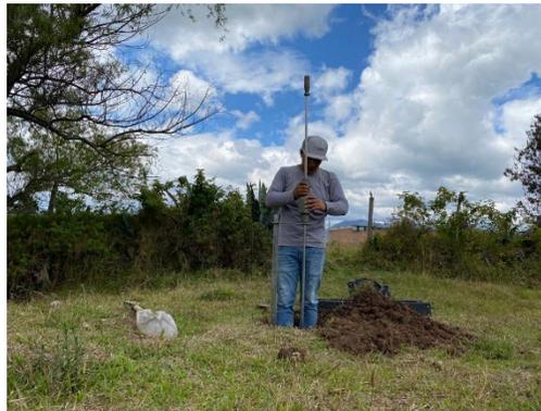
Fig. 5: DCP Test
