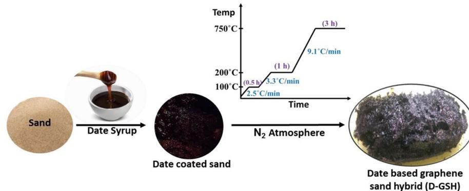
Figure 1: Synthesis process of D-GSH involves mixing sand with date syrup, then subjecting the mixture to a controlled N<sub>2</sub> atmosphere at accelerated temperatures until reaching 750°C, adopted from Khan et al. [12].
