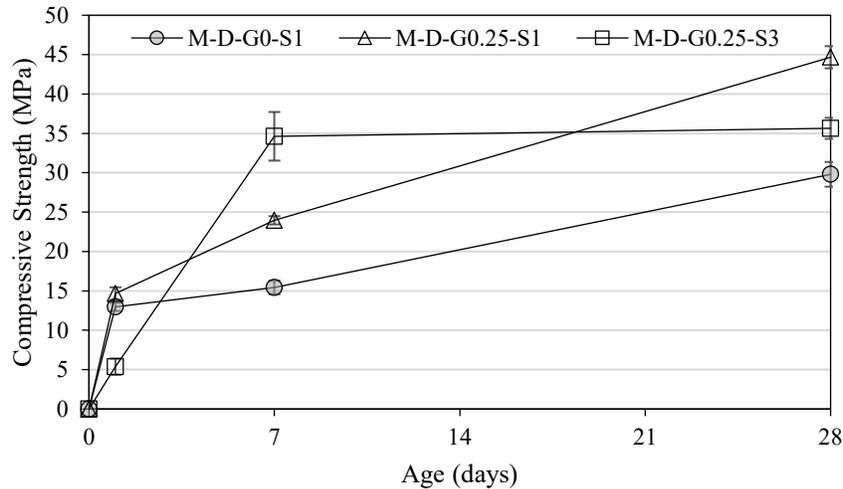
Figure 2: Compressive strength of mortar mixtures across time.
