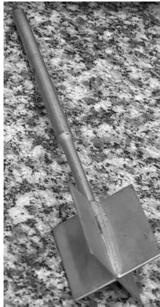
Fig. 3 Shear Vane used in the test setup
