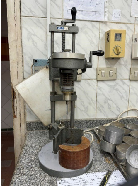
Fig.1: Laboratory Scale Shear Vane Apparatus
