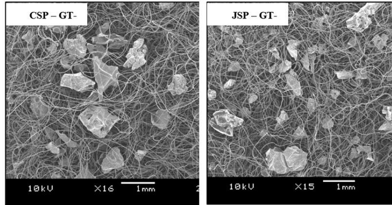
Fig. 12 SEM micrographs depict CSP (left) and JSP (right) infused GT-80 non-woven fabric, with a scale bar of 1 mm for reference.
