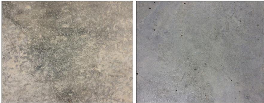
Fig. 14 Surface finish comparison: burlap-cured concrete (left) vs. innovative blanket (right).
