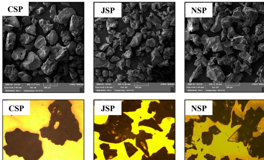
Fig. 7 SEM and optical micrographs of SAP powders: average particle sizes (top), various scales (bottom),  $500\mu\text{m}$  scale bar.
