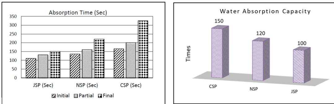
Fig. 9 Absorption time at different stages (left) and total capacity (right) for various SAP
