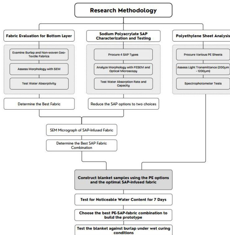
Fig. 1 Flowchart for Developing and Testing SAP-Infused Concrete Curing Blankets.
