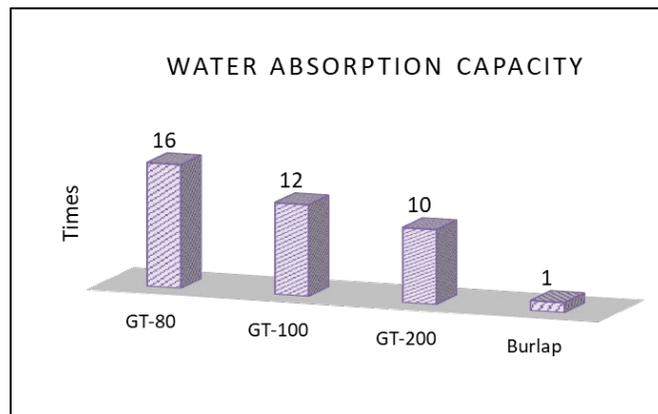
Fig. 11 Water absorption capacity of various fabrics relative to their weight.
