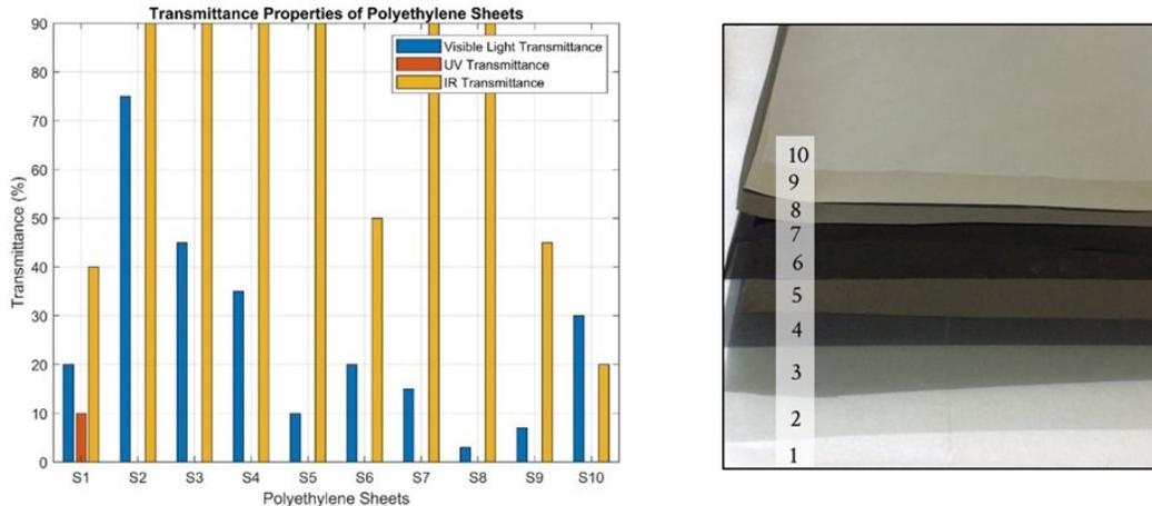
Fig. 2 Transmittance properties of polyethylene sheets, including VLT, UV, and IR, analyzed through spectrophotometer testing and wetting duration measurements.
