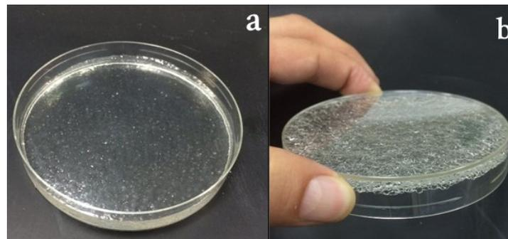
Fig. 3 Water Absorption Rate and Capacity Testing for SAP Variants. (a) Initial. (b) Final.
