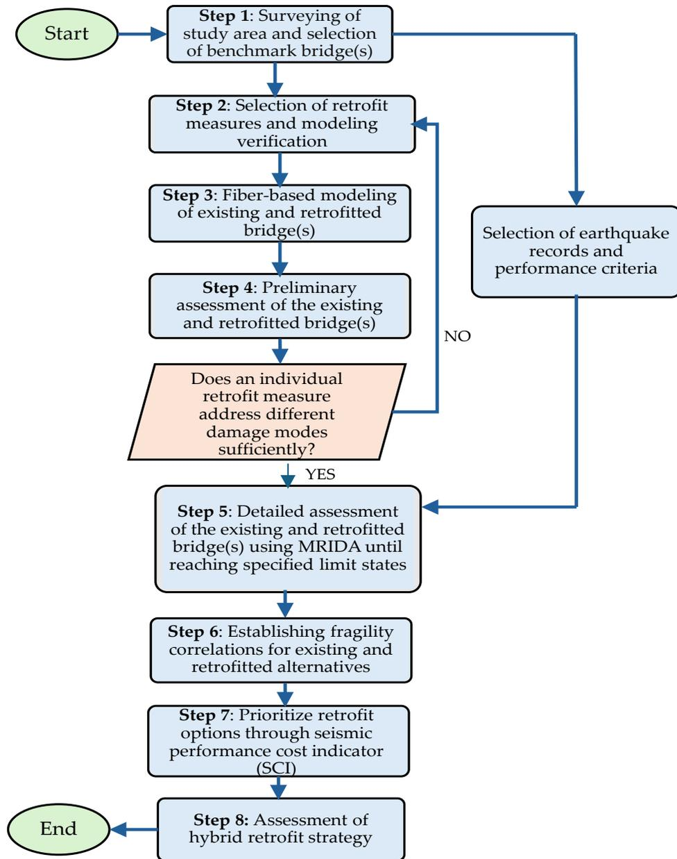
Fig. 3: The systematic methodology for upgrading existing substandard RC bridges.
