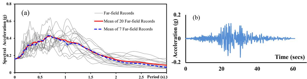
Fig. 1: Earthquake records normalized to the design intensity: (a) elastic response spectra of FF ground motions used for the seismic assessment; (b) acceleration history of a representative FF earthquake record.
