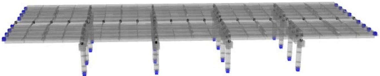
Fig. 2: Three-dimensional fiber-based numerical model of the reference bridge.
