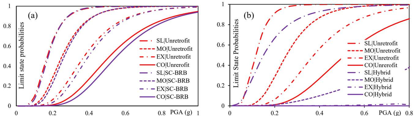
Fig. 4: Sample results of fragility functions for the un-retrofitted and retrofitted bridges pounding force demands under FF scenario: (a) effect of the individual retrofit measure, and (b) effect of the hybrid retrofit measure.
