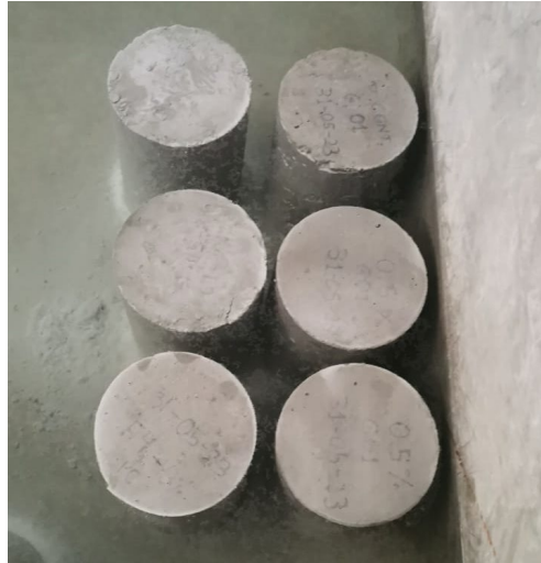
Fig. 2: Curing process of concrete test tubes fabricated.
