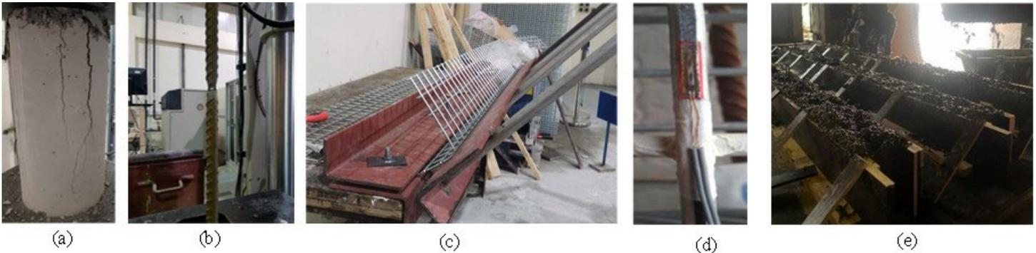
Fig. 2: Laboratory work, (a) concrete cylinder test, (b) steel bar test, (c) steel cage fabrication, (d) strain gauge, and (e) concreting.
