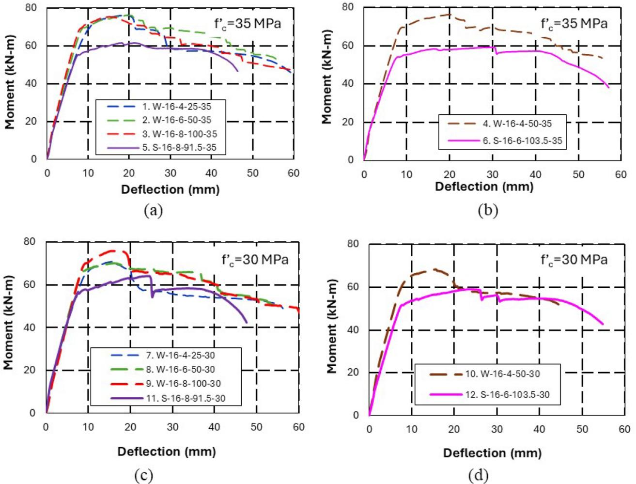
Fig. 4: Moment-deflection relationships, (a) Beams 1,2,3 & 5, (b) Beam 4 & 6, (c) Beams 7,8, 9 and 11, and (d) Beams 10 & 12.
