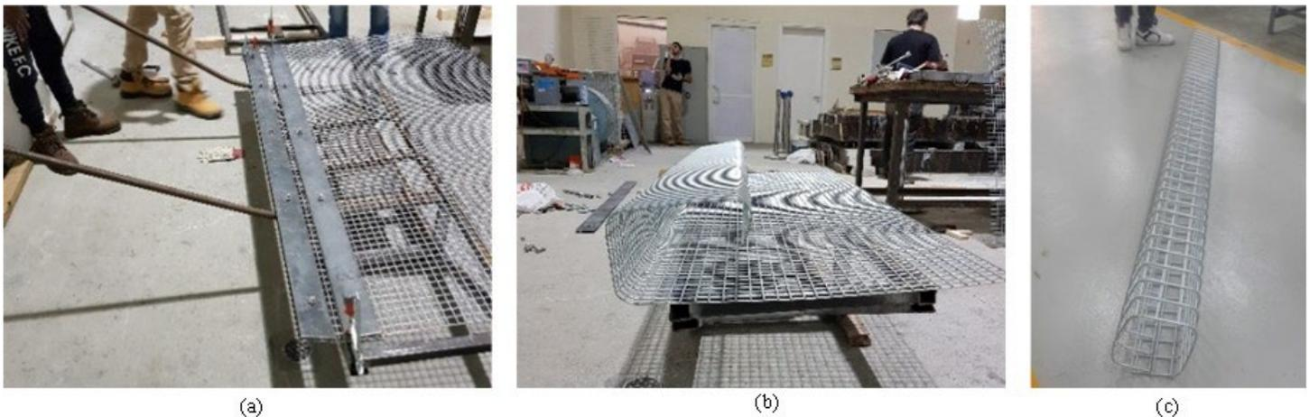
Fig. 1: Proposed use of WWR in concrete beams, (a) WWR setup for bending, (b) bending of the sheet, and (c) final product.
