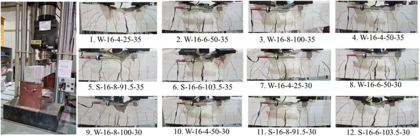
Fig. 3: Test setup and cracking pattern for all 12 tested concrete beams.
