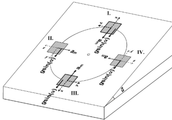
Fig. 5. Acceleration components during the rotation on an inclined plane
