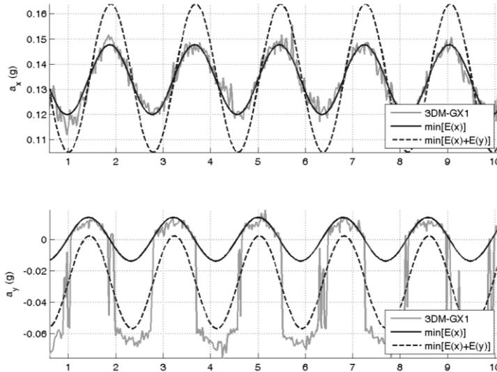
Fig. 8. Effect of different objective functions on the parameter estimation
