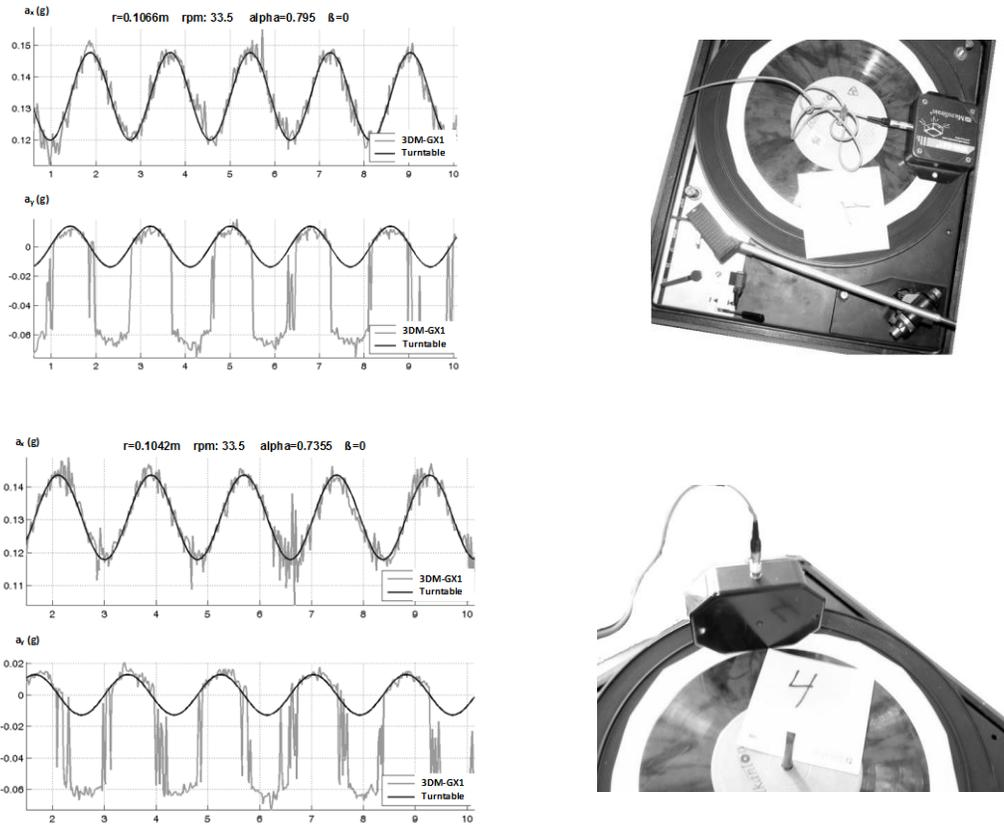
Fig. 9. Acceleration signals obtained from the model and received from the sensor
