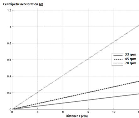
Fig. 3. The change of the centripetal acceleration with respect to  $r$
