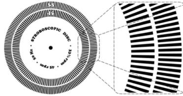
Fig. 2. Structure of the stroboscopic disc
