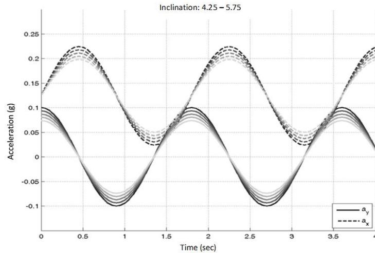
Fig. 6. Effect of the change in  $\alpha$  on  $a_y$  and  $a_x$ .
