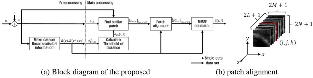
Fig. 1: Block diagram of the proposed method and the aligned similar patches in the main processing block.
